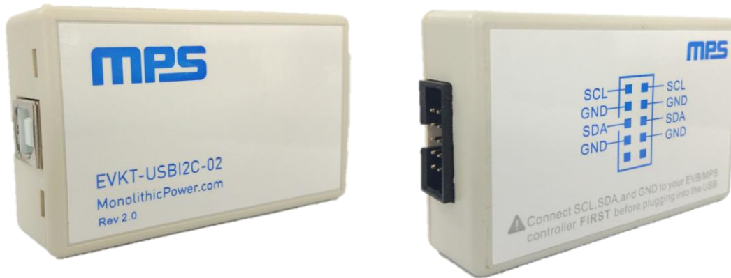
Figure 3: EVKT-USBI2C-02 Communication Interface
