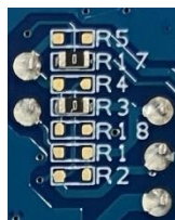
Fig. 4-3-1b I/O signal path around the PMIC and resistor lands
