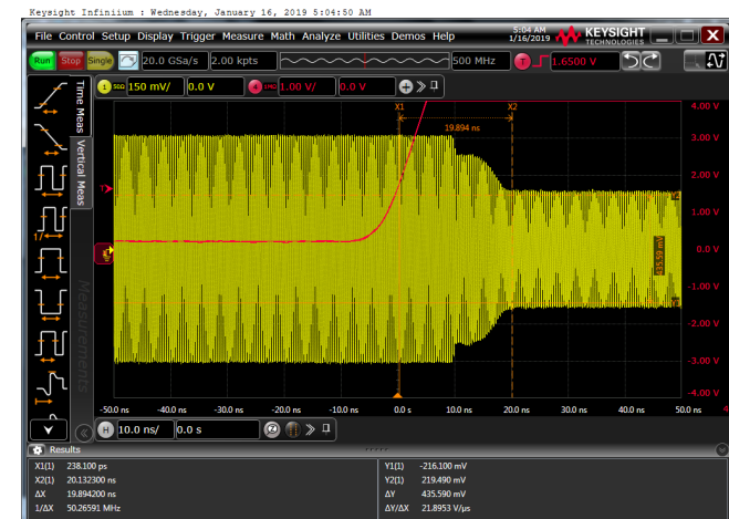
Figure 25. 6dB Gain Reduction Transient Time
