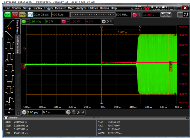
Figure 23. Standby to RX Mode Transient Time
