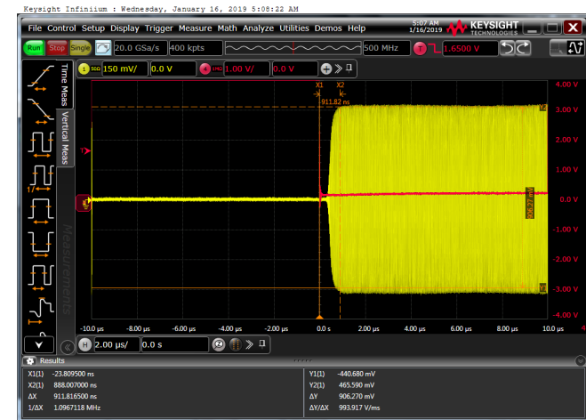
Figure 25. 6dB Gain Reduction Transient Time
