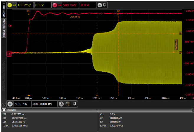
Figure 16. Switching Time Isolation to Insertion loss
