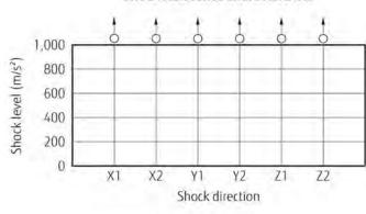
Shock application time: 11ms, half-sine wave Test material: coil energized and de-energized Shock direction: see diagram below Detection level: chatter > 100 µs
