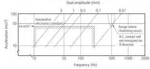
Frequency: 10~2000 Hz Acceleration: 100 m/s² max. Direction of vibration; see diagram below Detection level: chatter > 100 µs
