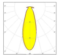
Dimensions: 85.0 mm x 85.0 mm Height: 23.00 mm ~25° beam for UV-C, warehouse and outdoor lighting. Compatible
