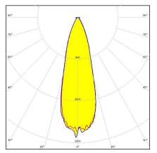
Dimensions: 90.0 mm x 90.0 mm Height: 39.15 mm ~25° spot beam. Compatible with up to 30 mm LES size COBs. Variant with black frame.
