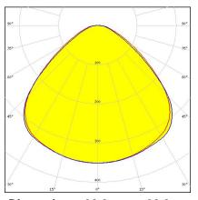
Dimensions: 90.0 mm x 90.0 mm Height: 11.30 mm ~100° very wide beam for warehouse and outdoor lighting.
