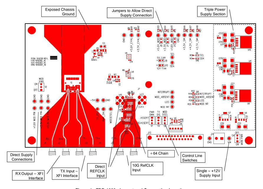
Figure 1. FDB-1022 - Layout and Connection Locations
