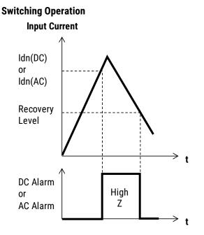
When the residual current exceeds the threshold level (Idn(DC) or Idn(AC)), PIN 4 (DC Alarm) or PIN 5 (AC Alarm) will change from low level to high impedance. Each output goes back from high impedance to low level when residual current falls below recovery level.
