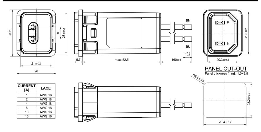
For dimensions [mm] without tolerances: ISO 2768-m / EN22768-m applies
