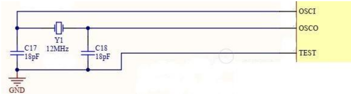
Figure 33 - Recommended FT2233HP/FT2232HP Crystal Oscillator Configuration
