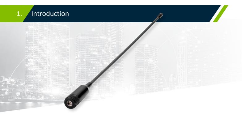
The Meteor FW.80 is a OdBi 169MHz ISM band 1/4 wavelength monopole flexible whip antenna with omnidirectional pattern optimized in the azimuth for wide coverage range in typical 169MHz applications such as Wireless M-Bus metering. It also finds its usage in remote asset monitoring applications, alarms, paging systems and private mobile radio services.
