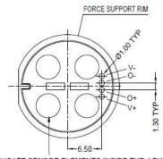
DELICATE SENSOR ELEMENTS INSIDE THE 4 BUMPS PROTRUDING 1.0MM MAX ABOVE RIM, DO NOT APPLY ANY FORCE.
