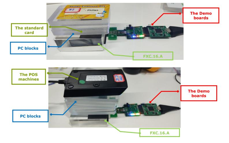
When the number of the PC material blocks are carefully adjusted until the reader can no longer read the sample, that's mean in this point the FXC.16.A cannot establish communication with the standard card or the POS machine, the thickness of the PC material block is the maximum interrogation distance of them.
