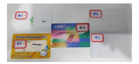
Type 1 is based on ISO/IEC 14443A standard and has 96 bytes of memory.
