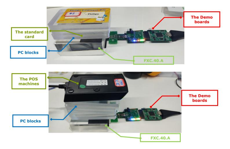
When the number of the PC material blocks are carefully adjusted until the reader can no longer read the sample, that's mean in this point the FXC.40.A cannot establish communication with the standard card or the POS machine, the thickness of the PC material block is the maximum interrogation distance of them.
