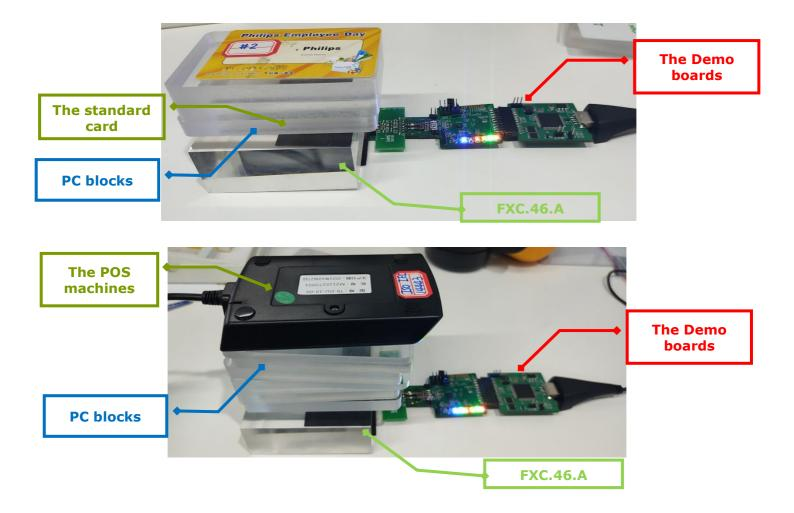
When the number of the PC material blocks are carefully adjusted until the reader can no longer read the sample, that's mean in this point the FXC.46.A cannot establish communication with the standard card or the POS machine, the thickness of the PC material block is the maximum interrogation distance of them.
