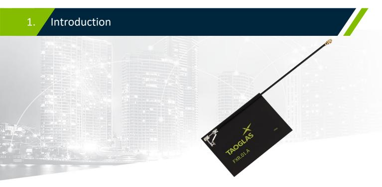
Taoglas has developed an NFC (Near Field Communications) antenna for use with NFC readers. This standard design is matched to a 50 Ohm system and provides a well-matched solution for NFC readers. The antenna is dimensioned to provide the capability of interrogating typical size NFC tags out to a 5 cm. distance. This standard antenna is delivered with a coaxial cable connected to the antenna element to ease use and integration into customer devices.
