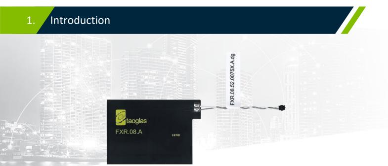
The FXR.08.52.0075X.A.dg is an NFC Ferrite antenna with 75mm twisted pair 28AWG cable and JST connector. It works with specific NFC chips which need to connect via JST ACH connector.
