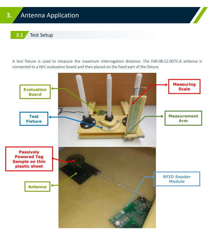
The test sample is placed on a thin sheet of plastic connected to the movable part of the fixture. Then the distance is carefully adjusted until the reader can no longer read the sample, thus the maximum interrogation distance is displayed in the ruler.
