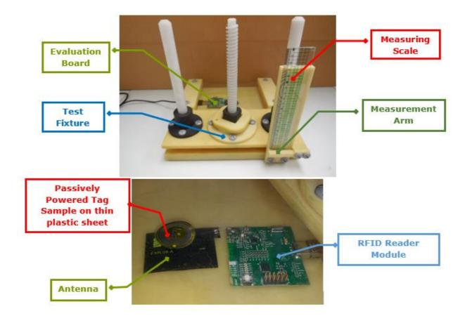
The test sample is placed on a thin sheet of plastic connected to the movable part of the fixture. Then the distance is carefully adjusted until the reader can no longer read the sample, thus the maximum interrogation distance is displayed in the ruler.
