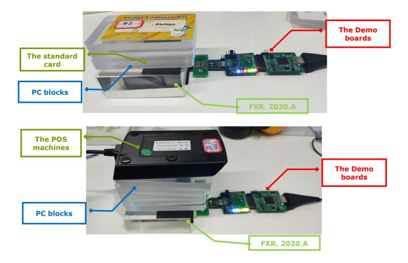
When the number of the PC material blocks are carefully adjusted until the reader can no longer read the sample, that's mean in this point the FXR.2020.A cannot establish communication with the standard card or the POS machine, the thickness of the PC material block is the maximum interrogation distance of them.
