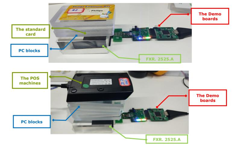
When the number of the PC material blocks are carefully adjusted until the reader can no longer read the sample, that's mean in this point the FXR.2525.A cannot establish communication with the standard card or the POS machine, the thickness of the PC material block is the maximum interrogation distance of them.
