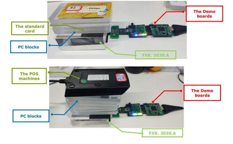
When the number of the PC material blocks are carefully adjusted until the reader can no longer read the sample, that's mean in this point the FXR.3030.A cannot establish communication with the standard card or the POS machine, the thickness of the PC material block is the maximum interrogation distance of them.
