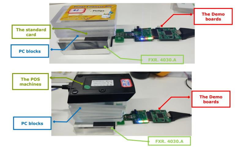
When the number of the PC material blocks are carefully adjusted until the reader can no longer read the sample, that's mean in this point the FXR.4030.A cannot establish communication with the standard card or the POS machine, the thickness of the PC material block is the maximum interrogation distance of them.
