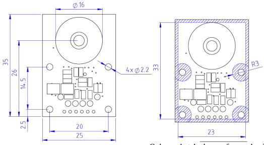
Only use hatched areas for mechanical assembly (screws, nuts, etc).
