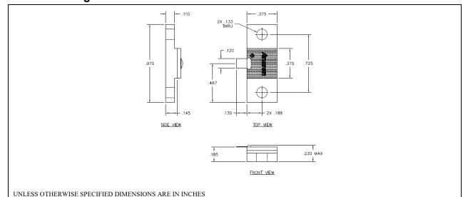
Tolerance is ±0.010", unless otherwise specified. Designed to meet or exceed applicable portions of MIL-E-5400. All dimensions in inches.
