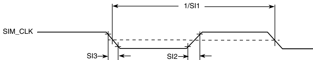
Figure 50. USIM Clock Timing Diagram
