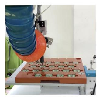
Please note that this process will require a one-time fixture to be made for each PCB design, Example as per image above.
