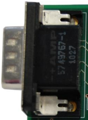
Figure 2.3: 15-pin VGA connector for power supply
