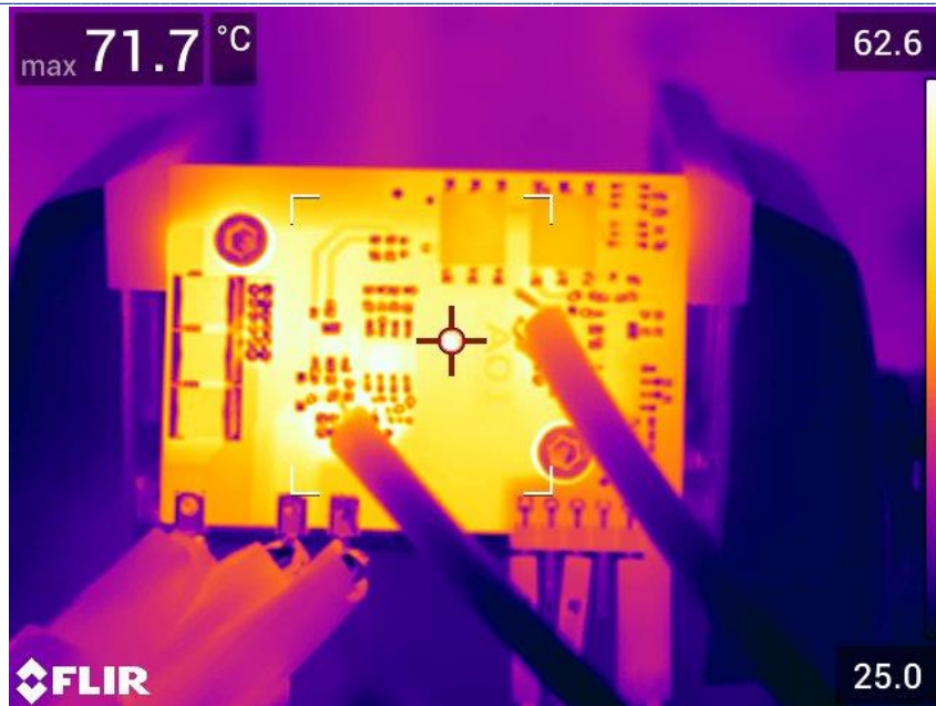
Figure 12 Boost configuration test thermal measurement result
