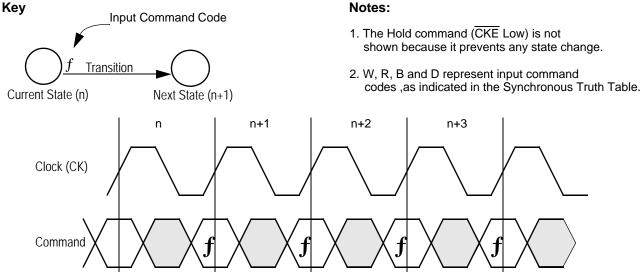
Current State and Next State Definition for Pipeline and Flow Through Read/Write Control State Diagram
