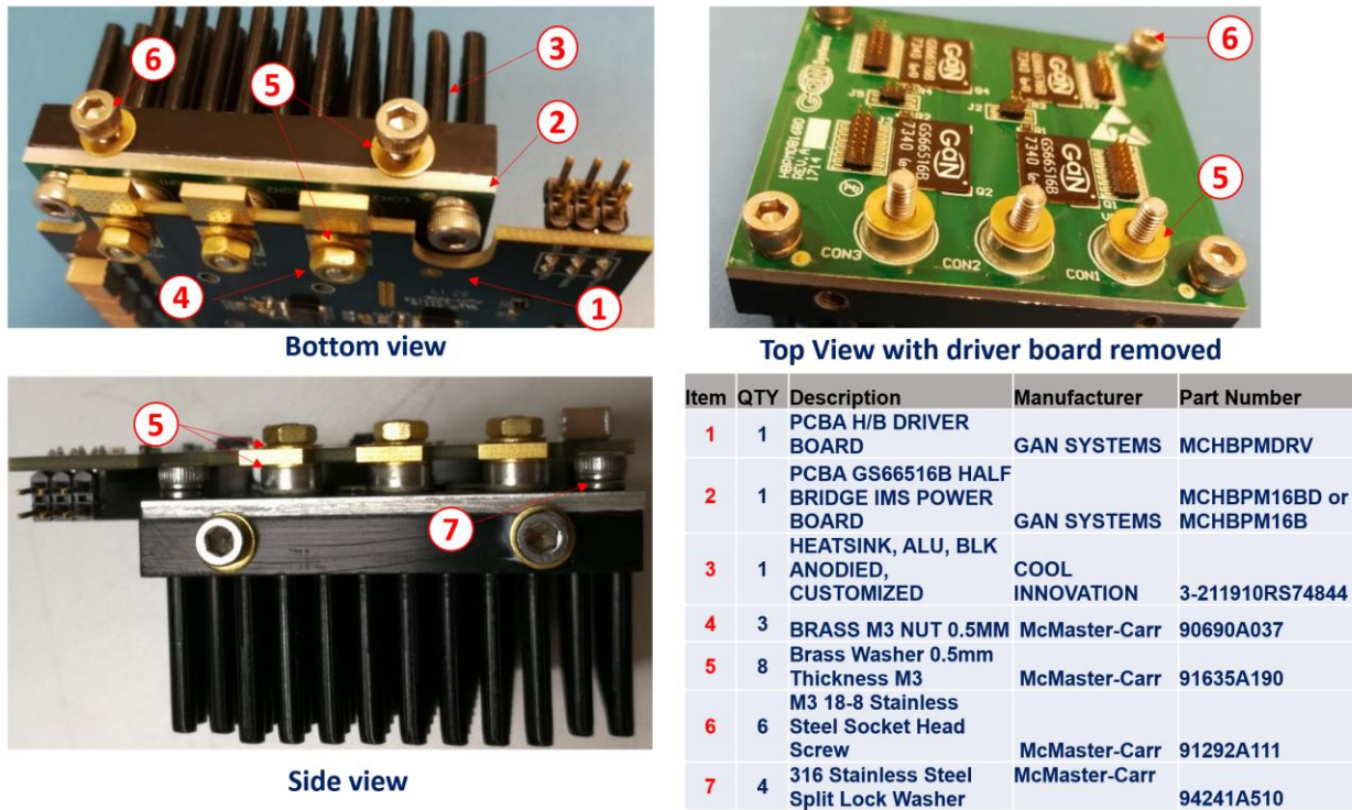
Figure 10 - IMS evaluation module assembly
