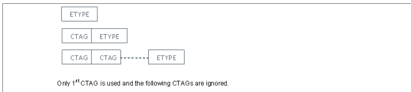
Figure 30 Supported Frame Formats when STAG is disabled
