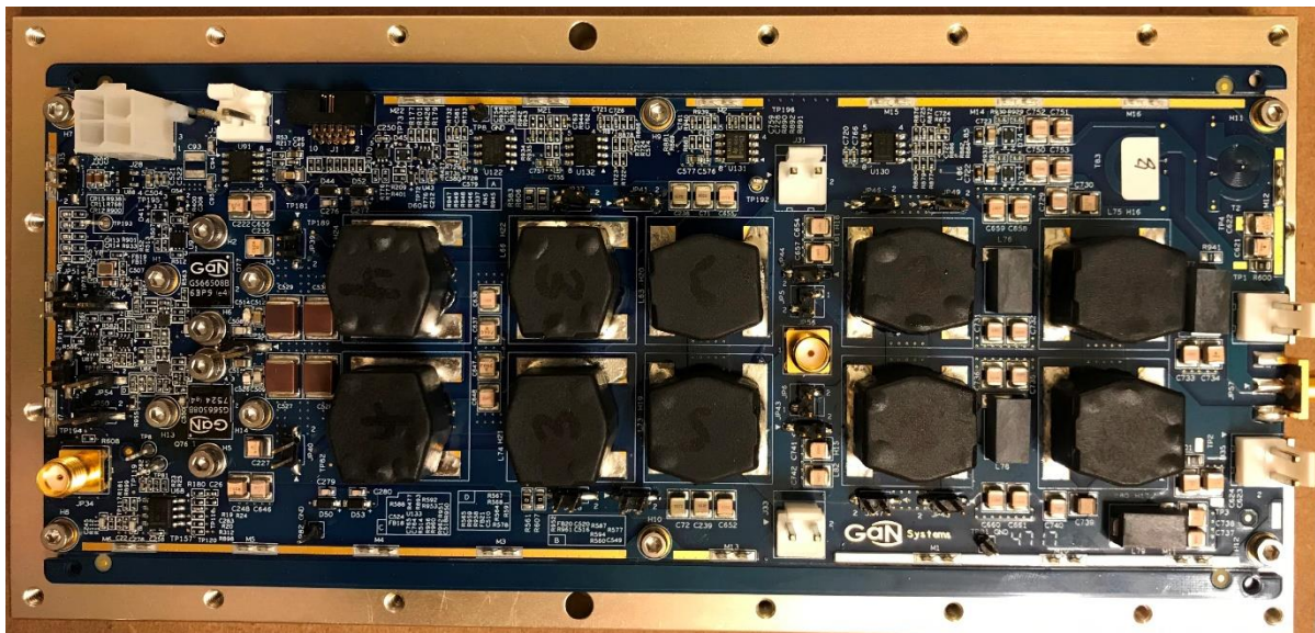
Figure 2 • Top side of GSWP300W-EVBPA Evaluation Board Assembly
