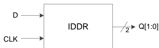
Figure 3-16 I/O Logic in DDR Input Mode
