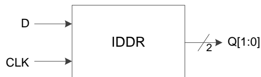
Figure 3-16 I/O Logic in DDR Input Mode
