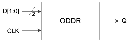
Figure 3-17 I/O Logic in DDR Output Mode
