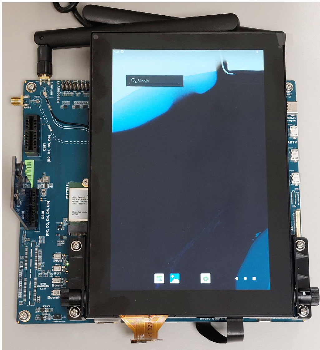
Figure 2-1. Genio 700 EVK Board System Setup
