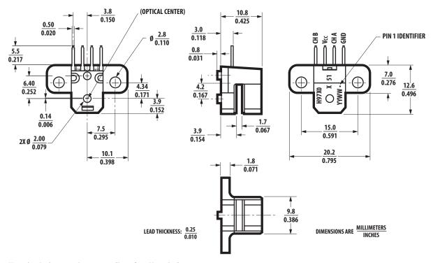
Mounting Option #51 – Screwmount (Baseplane Mounting)
