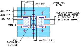
NOTES: 1. COPLANAR WAVEGUIDE PARAMETERS ARE SHOWN FOR ROGERS R04350B WITH THICKNESS .020"  $\pm$  .0015". COPPER: 1/2 OZ. EACH SIDE. FOR OTHER MATERIALS TRACE WIDTH & GAP MAY NEED TO BE MODIFIED.
