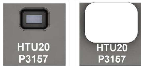
Laser marking on HTU20P(F) sensor
