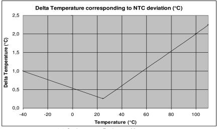
0.1°C tolerance on Resistance Measurement
