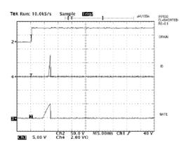
For most applications and pass elements, the HV100 provides adequate limiting of the maximum current to prevent damage without the need for any external components. The 2.5s delay of the auto-retry circuit provides time for the pass element to cool between attempts.
