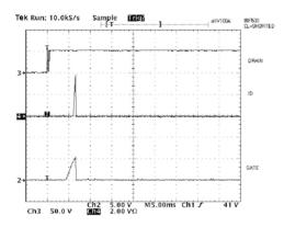
The maximum current that may occur during this period can be controlled by adding a resistor in series with the source of the MOSFET. The lower graph shows the same circuit with a 100m $\Omega$  resistor inserted between source and VNN. In this case the maximum current is 25% smaller.
