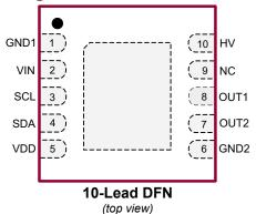
Pads are at the bottom of the package. Center heat slug is at ground potential
