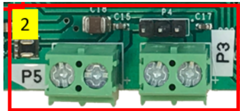
Figure 3 - 12 V power supply connection
