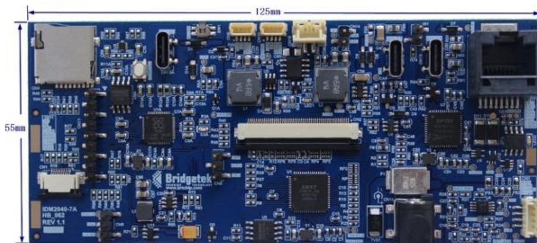
Figure 13 – IDM2040-7A Board PCB Dimensions (Top View)
