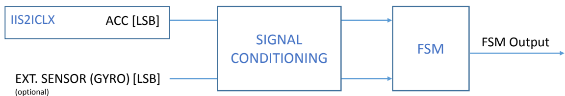
Figure 2. State machine in the IIS2ICLX
