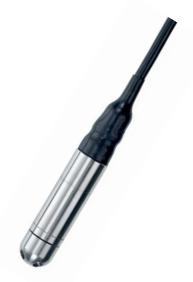
The ILS is designed for use in continuous submersion in liquids such as water, oil and other non-aggressive chemicals. The submersible uses the latest piezo-resistive media-isolated silicon sensing technology and a stainless steel diaphragm within a 316L stainless steel housing.
