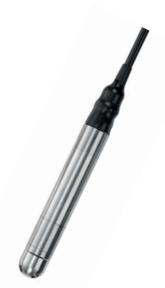
The ILTSU is designed for use in continuous submersion in liquids such as water, oil and fuels. The probe uses the latest piezoresistive media-isolated silicon sensing technology and a stainless steel diaphragm. Housed within a 316L stainless steel, or high grade Duplex stainless steel housing, this submersible transmitter is the ideal product for hydrostatic level measurement where temperature is also a critical part of
