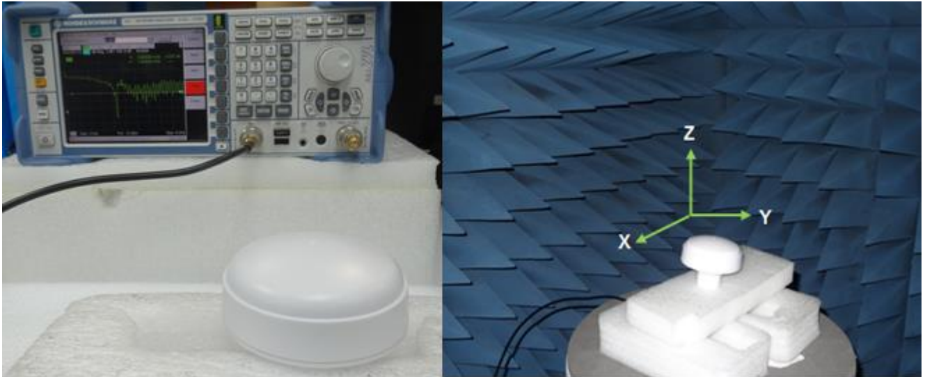
Figure 1. Impedance (left hand), Efficiency, peak gain, and radiation pattern measurements (right hand).
